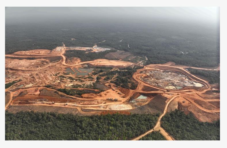
Only Open-Pit Operations are ongoing at this site. Three different open pit are located. (Matambo-1, Matambo-2, Matambo-3) Ore production from open-pit operations started at the end of 2023 with all the ore being transported to the New Liberty processing plant.
