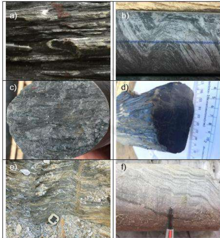
a) F1 isoclinal fold hinges attributed to remnant transposed layering during D1; b) F2 folds with weakly developed S2 foliations AXPL to folds; c) L21 intersection lineation; d) Rod-shaped L-tectonite fold hinge structure of F2 fold axis; e) Open gentle F3 folds with weakly developed spaced AXPL cleavage; f) Weakly developed F3 crenulation cleavage.
