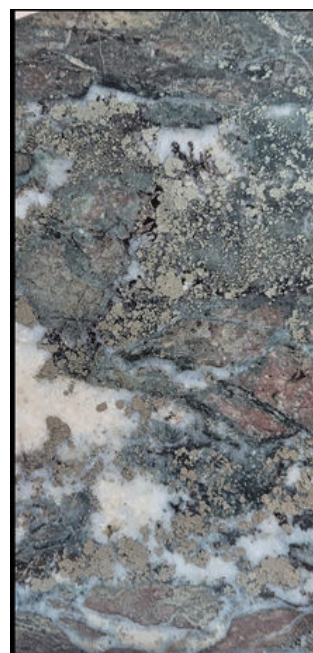
A photo of gold mineralisation from GRE46. Quartz (white) pyrite (brassy) and sphalerite (black) in a diorite rock.
