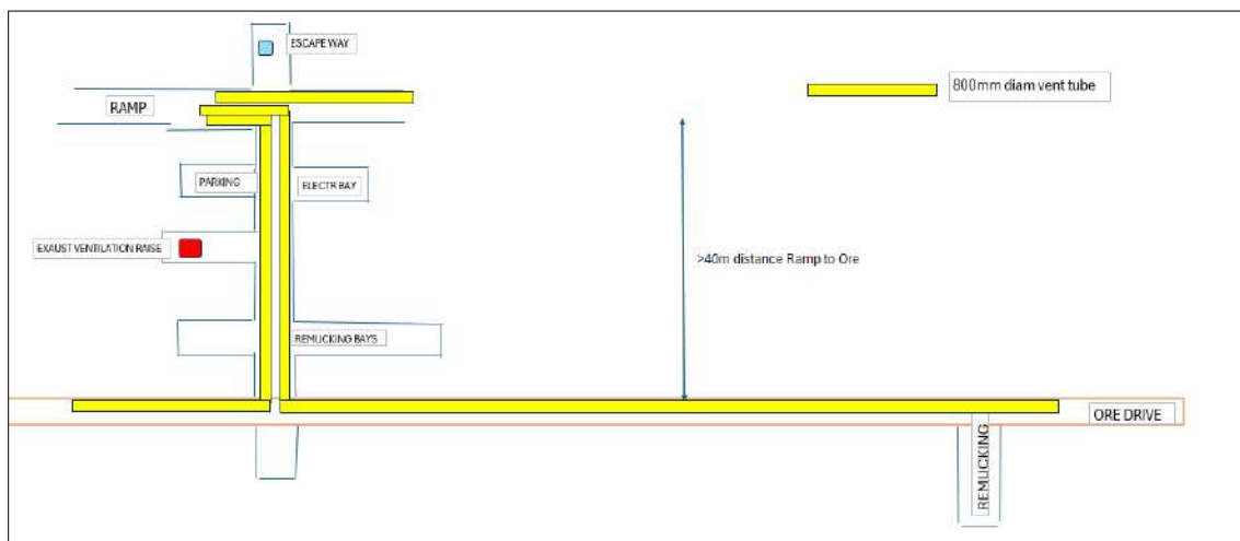
Figure 16.18: Secondary Ventilation System.
