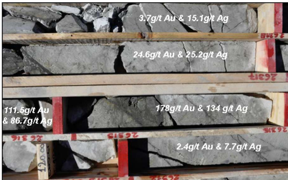
Figure 7.15: Core mineralised intervals, CND123
