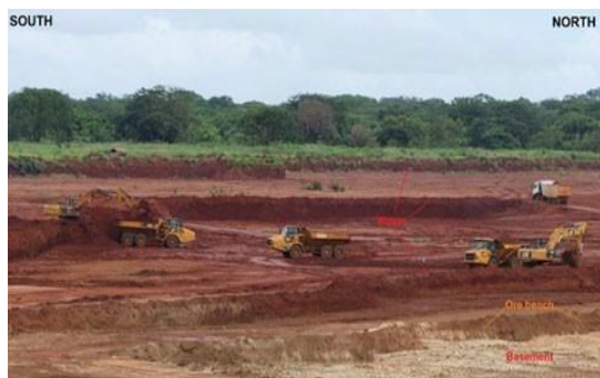
Figure M11: Systematic and selective mining under Geology supervision.
