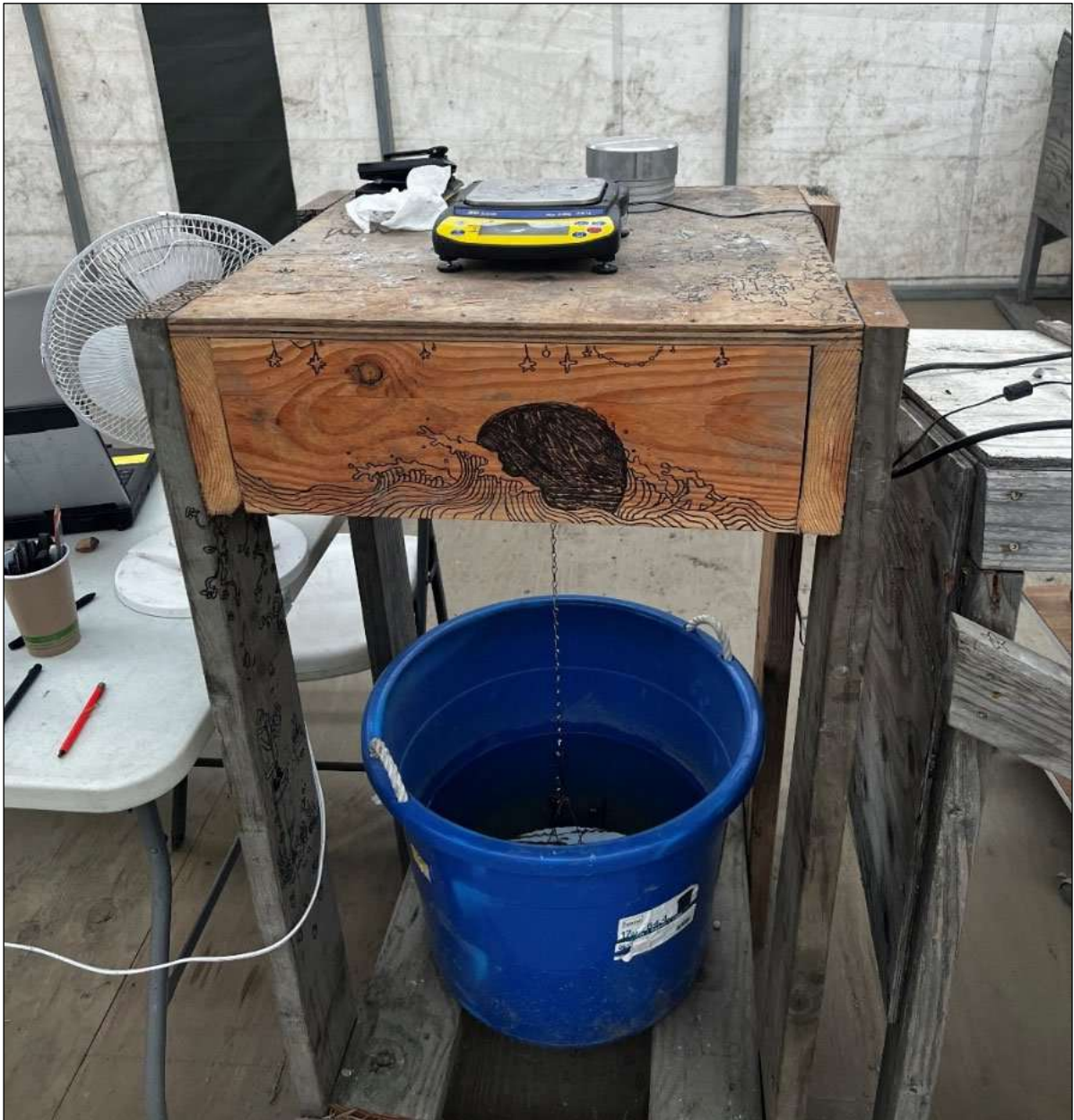
Figure 10-4: Specific Gravity Measurement Setup at Palmer
