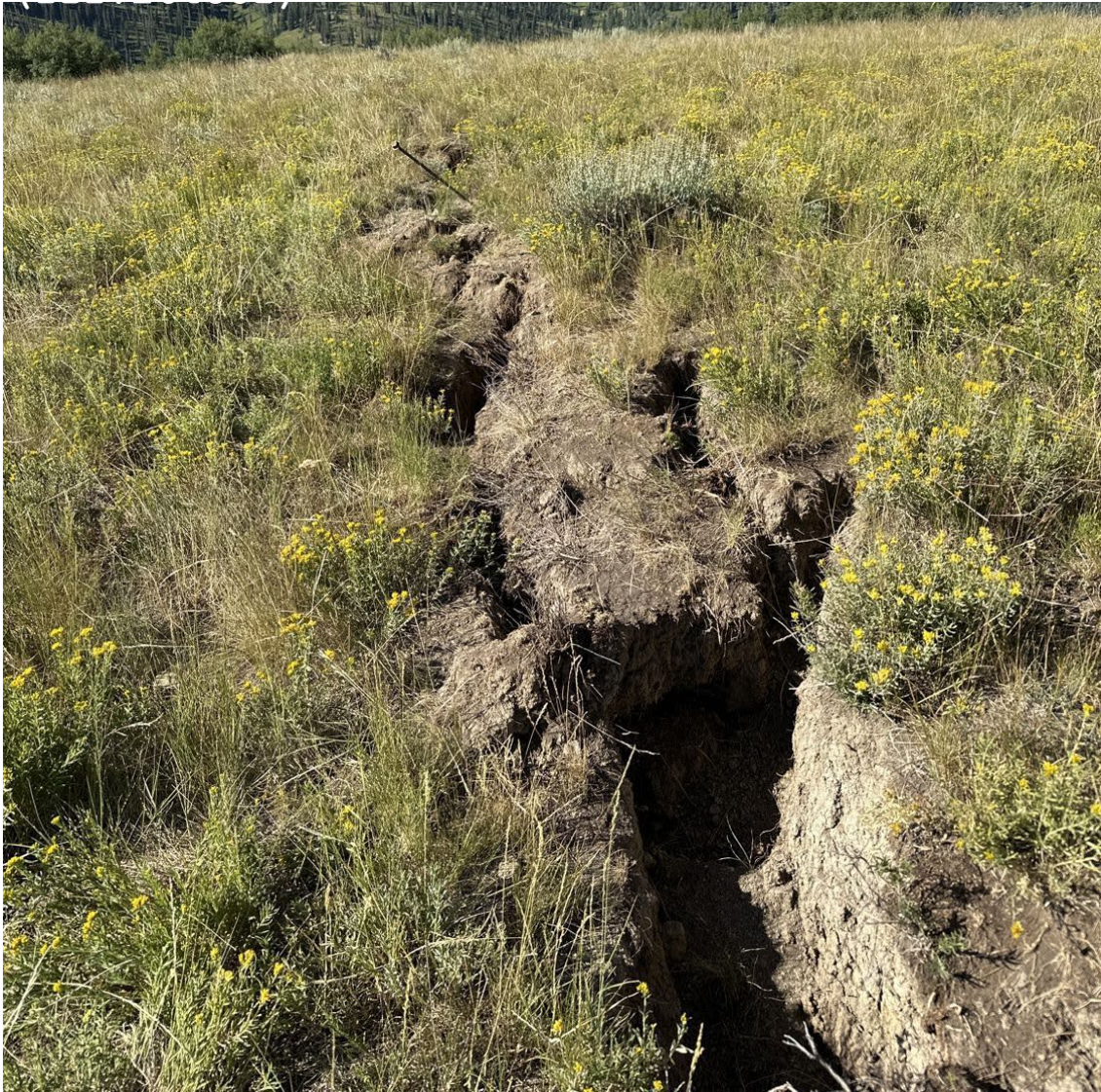
Figure 3.6–3. Typical Tensile Fracture Resulting from Subsidence Affecting Mountain Shrubland Vegetation Community
