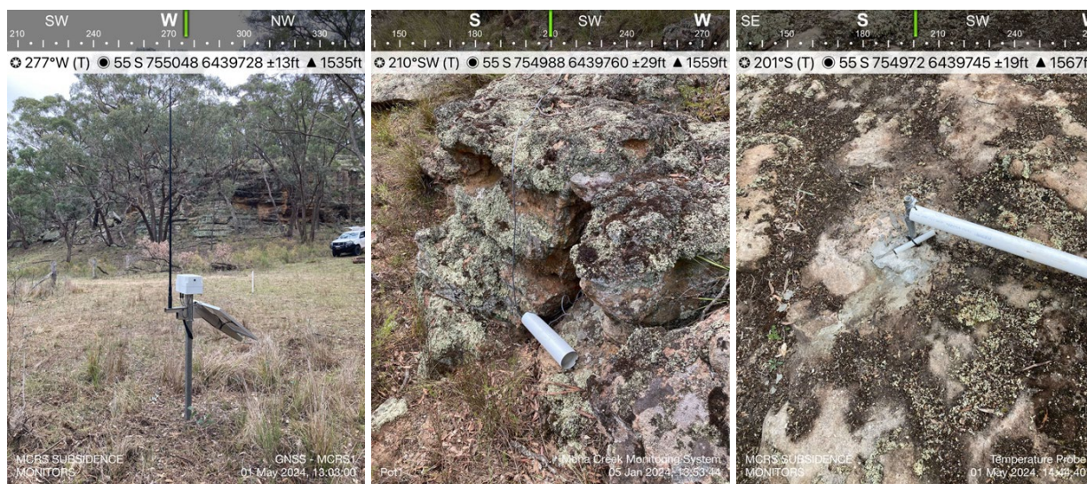
Photo 4 Example of a GNSS & Potentiometer Units within the MCRSS
